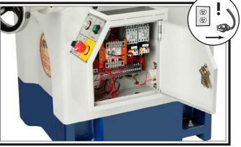
Figure 60. Electrical box & control panel location.
